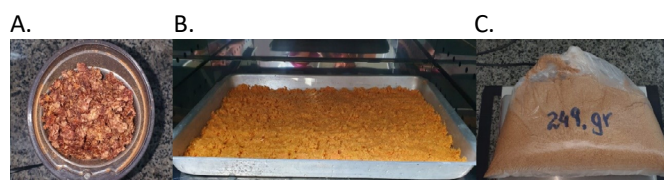
Figure 1. Acerola bagasse residue (A) before drying, (B) after drying and (C) after drying and grinding - FRA.
