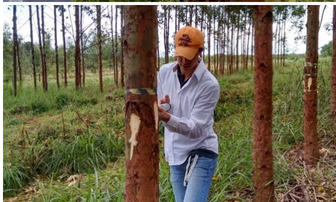
Figure 2. Use of a Pilodyn meter to determine the density of wood from Eucalyptus grandis x Eucalyptus urophylla trees planted at Embrapa Agrossilvipastoral, in Sinop, Mato Grosso, Brazil.
