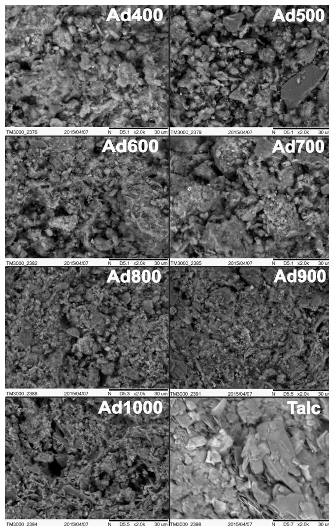
**Figure 1.** Electron micrographs obtained by scanning electron microscopy of the adsorbents prepared from the sewage sludge (Ad400 to Ad1000) and talc.
