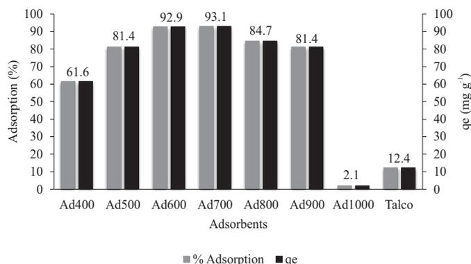
**Figure 6.** Percentage of adsorption of wood extractives and adsorption capacity ( $q_e$ ) for the adsorbents.
