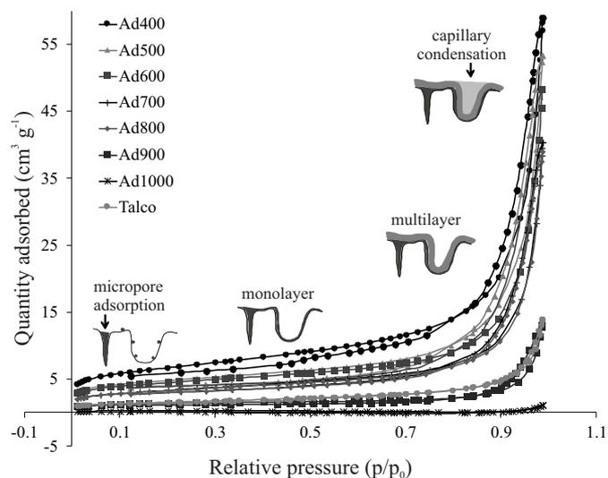
**Figure 2.** Nitrogen adsorption and desorption isotherms of adsorbents Ad400 to Ad1000 and talc.
