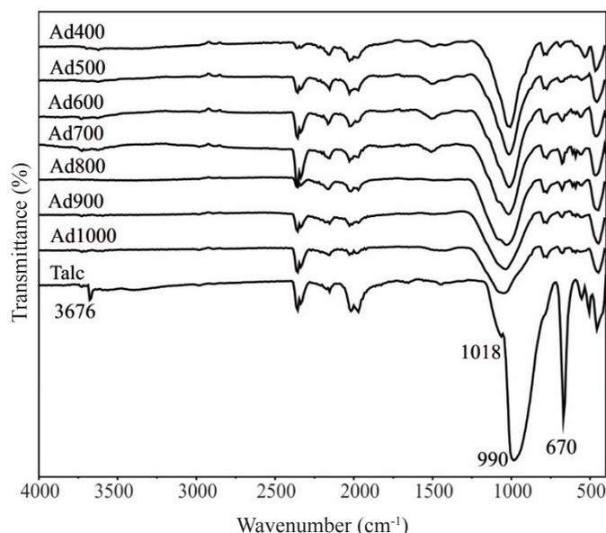
**Figure 4.** Fourier transformed infrared spectroscopy (FTIR) spectra of the adsorbents and talc.
