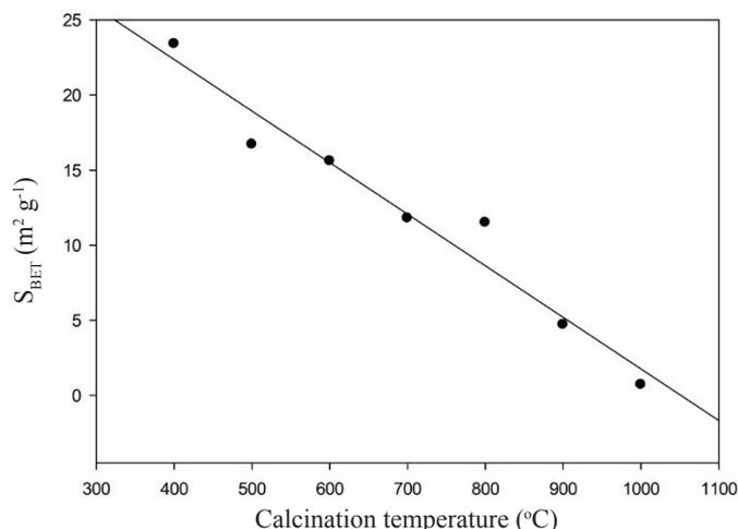
**Figure 3.** Influence of the calcination temperature on the  $S_{\text{BET}}$  values (specific surface area).
