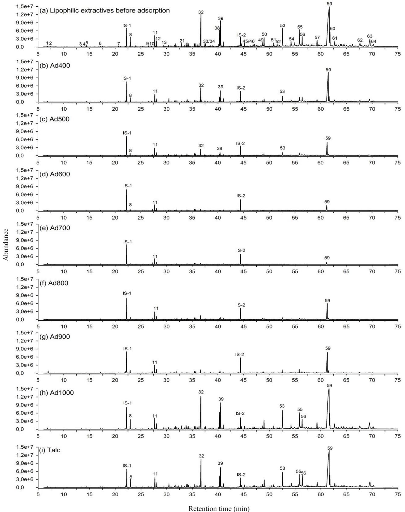
IS-1 and IS-2: Internal standards: hexanedioic acid and tetracosane, respectively.
