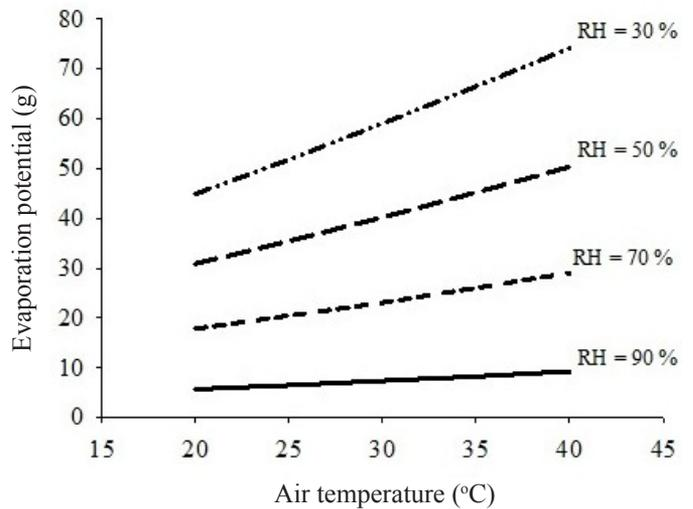
Figure 2. Water evaporation potential of the climate chamber as a function of temperature and distinct values of relative humidity (RH).
