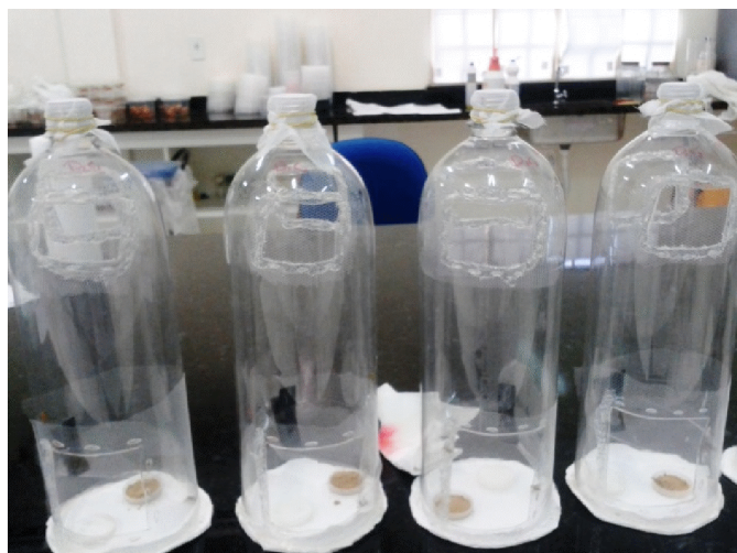
Figure 2. Cages made from 2-liters polyethylene terephthalate (PET) bottles to observe the sexual behavior of A. striata
